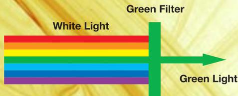
Most artificial light sources do not actually produce white light. For example, incandescent sources such as tungsten generate light which has more energy at the red end of the spectrum, whereas a fluorescent source often has spikes of energy mainly in the blue and green region. Filters can be used to correct these differences and make one light source appear like another.
