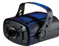
The X-Effects Projector provides large scale 3-D effects previously unavailable to lighting designers. The device utilizes a 200-watt Enhanced Metal Arc source, whose short arc allows for an output of 5000 lumens, and a 7000 hour lamp life. The colour temperature is similar to a Xenon source at 6000°K, but with nearly two times the luminous effectiveness.
